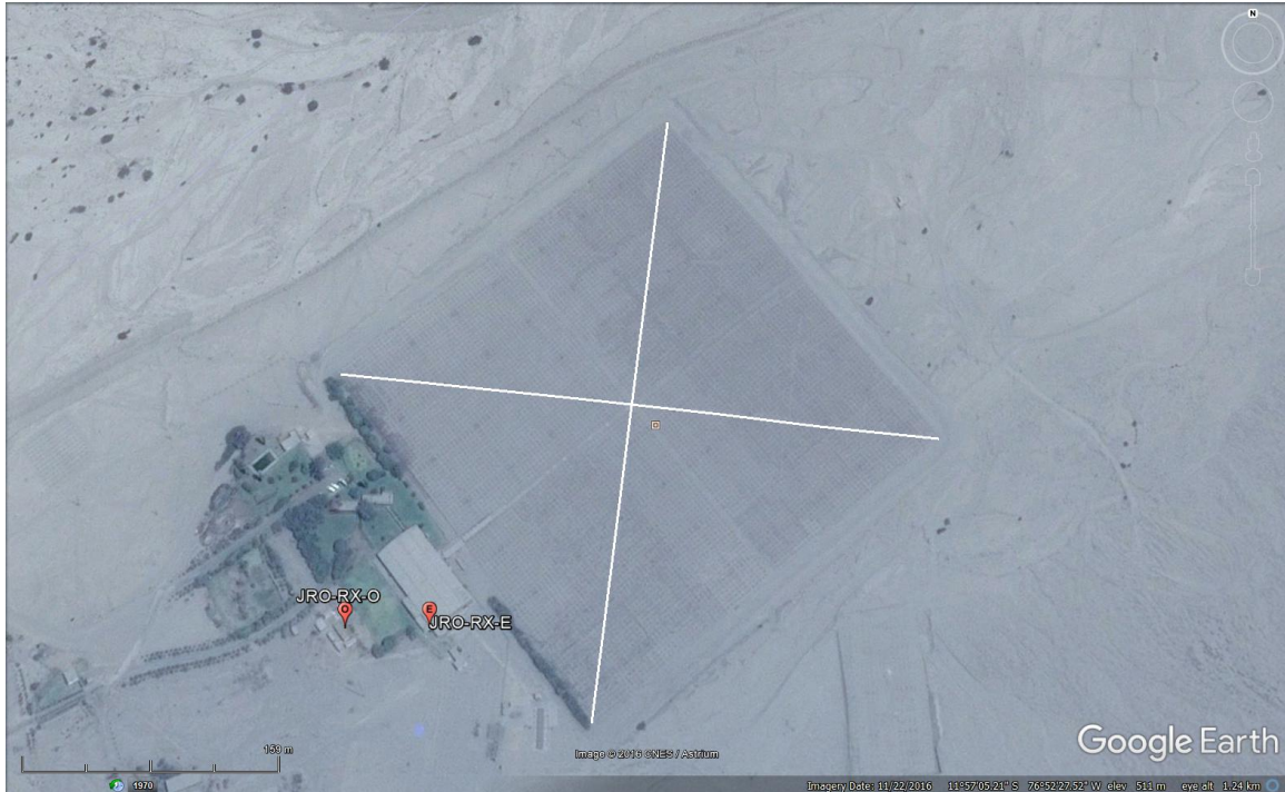
Figure 2.5. The radar array at Jicamarca Radio Observatory, Peru at 11.95^\circ S, 76.87^\circ W with inclination 1.145^\circ and declination 0.367^\circ . The magnetic field line is nearly horizontal. The receiver pair O,E is also shown as tiny red pins, whose baseline points in the geomagnetic east-west direction nearly parallel to the local field line in white. Courtesy of Google Maps.
