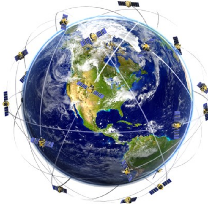
Figure 1.1. A Global Navigation Satellite System (GNSS) is a constellation of satellites (space segment) and users (ground segment). Image credit [3].
