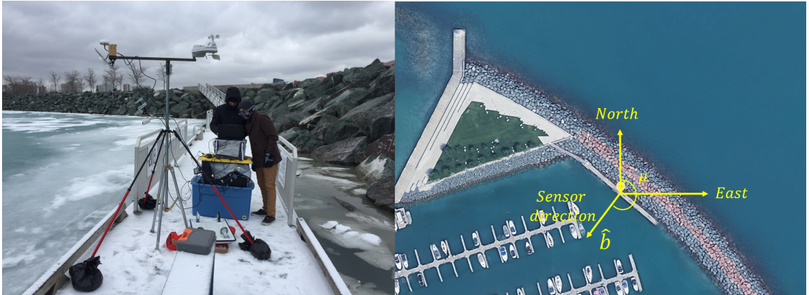
Figure 4.3. Left: Photo of the experiment hardware setup for Test 1-East. Right: Google Map satellite image of sensor location for Test 1-East. The yellow arrow describes the boom direction \hat{b} .
